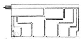
With a V-shaped arrangement of explosive filled grooves the minimum allowed distance as a function of time difference between a detonating trace and neighboring later detonating trace can be continuously measured and analyzed.
