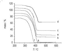
$a-d_{50} = 0.30 \mu \text{m}$ ,  $b-d_{50} = 1.16 \mu \text{m}$ ,  $c-d_{50} = 2.05 \mu \text{m}$ ,  $d-d_{50} = 3.40 \mu m$ ,  $e-d_{50} = 0.76 \mu m$ ,  $f-d_{50} = 0.46 \mu m$
