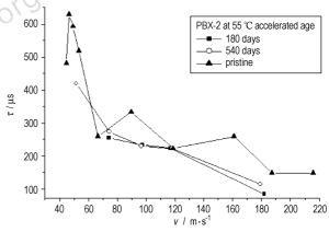
PBX-2 explosive for 55 °C accelerated age 180 days and 540 days are tested in Steven test by using a steel projectile of 2.0 kg. In the test the reaction overpressures are gained by blast pressure gauges. The results primarily show that there is not obvious change for the reaction degree of pristine and accelerated aged PBX-2 explosive in Steven test.
