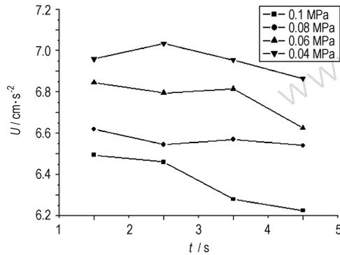
**Fig. 2** Relation between expanding velocity of pyrotechnic smoke cloud ( $u$ ) and times ( $t$ ) under different vacuum pressure
