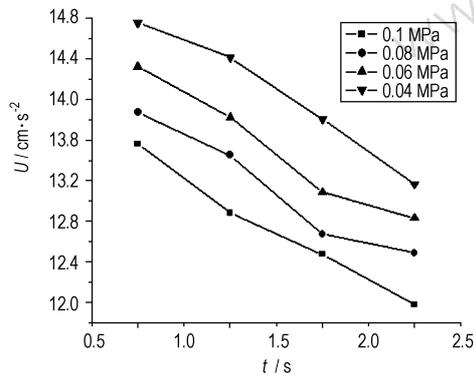
Fig. 3 Relation between expanding velocity of powder smoke cloud ( $u$ ) and times ( $t$ ) under different vacuum pressure
