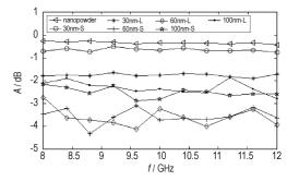
With the static measuring method, the microwave attenuation performances of carbon nano-powder, carbon nanotubes, and carbon nanofibers were studied. The average attenuation values per quality density for 7 kinds of carbon nano-materials with different structures and sizes were given.
