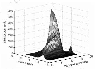
The infrared extinction of super-fine ceramic fiber coated nickel was studied with numerical simulation and experimental measurement. The rules were researched that extinction property of fiber changed with wavelength, aspect ratio of fiber, conductivity, refractive index, and dielectric constant. The extinction coefficients were compared between metal coated fibers and uncoated fiber.
