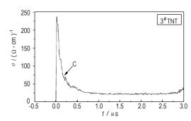
The typical electrical conductivity profile was obtained in the shock initiation process of TNT explosive by scheme of planar measurement.
