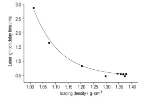
YAN Nan, ZENG Ya-qin, FU Hong Chinese Journal of Energetic Materials, 2008, 16(5): 487-489 Laser ignition delay time of Zr/KClO<sub>4</sub> over a large range of loading pressures or charge densities was studied. The high precision relationship between ignition delay time and density was obtained.
