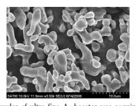
The mould powder of ultra-fine A5 booster was acquired by aqueous suspension technology. The component and pattern of ultra-fine A5 booster were ZHANG Jing-lin, JIANG Xia-bing, characterized by FT-IR and SEM. Comparison between ultra-fine A5 and commercial A5 by impact sensitivity, shock wave sensitivity and energy Chinese Journal of Energetic Materials, 2008, 16(5): 515-518 output were carried out.
