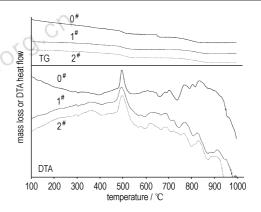
Three kinds of tungsten type delay compositions were tested by TG-DTA method to investigate the effects of nano-Fe, O<sub>3</sub> on combustion properties.
