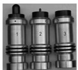
Steven test for PBX-2 explosive was made by using different shape warhead steel projectiles of 2.0 kg. PVDF pressure gauges were added for pressure
