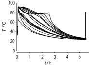
Multiple channels data collecting instrument has been used to investigate the temperature distribution of the melt-cast explosive during the cooling process under various cooling conditions.
