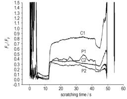
The friction properties of two types of polymer bonded explosives coded P1 and P2 and two coatings named C1 and C2 have been tested by the universal testing machine based friction system and the nano-indenter respectively.
