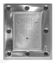
HAN Jun-qi, MENG Zi-hui, MENG Wen-jun, CHEN Guang-wen, WANG Bo-zhou, GE Zhong-xue Chinese Journal of Energetic Materials, 2010, 18(1): 34-36 Nitrate ester explosives were synthesized in chip based micro reactor. When alcohol and nitric-sulfuric mixed acid are mixed in the micro reactor, the yield of EGDN is 86.4%, and the yield of diethylene glycol dinitrate is 90.6%.
