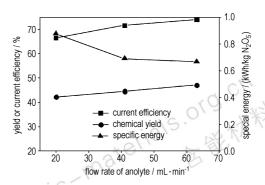
Dinitrogen pentoxide was prepared by the electro-oxidation of tetroxide dinitrogen in anhydrous nitric acid on the RuO<sub>2</sub>-IrO<sub>2</sub>/Ti anode.
