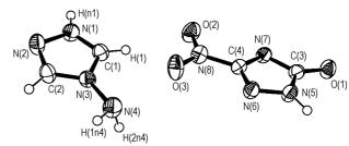
A new energetic salt 4-amino-1,2,4-triazole NTO salt was prepared and characterized by X-ray diffraction ometer, and its sensitivity and thermal properties were obtained.
