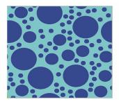
A representative volume element (RVE) of compostion B explosive was established in which the rounds were RDX grains that were periodic on the boundaries, and the other part is TNT. By using the RVE model, the effective elastic properties including elastic modulus and Poisson's ratio were predicted.
