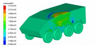
3D simulation of an armored vehicle model composed of 4340 steel and rubber was performed by AUTODYN software. The explosion process of 8701 explosive under different charge mass conditions was calculated. The response parameters of three observation points on the side such as overpressure, displacement and acceleration were obtained. The regularity of dynamic response for the observation points was analyzed.
