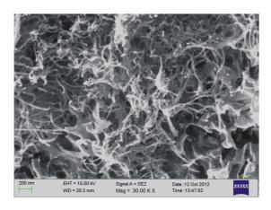
A kind of antistatic nitrocellulose membrane was prepared by adding conductive filler to the nitrocellulose. Scanning electron microscope images reveal that some interlaced conductive networks were formed, which result in the electrostatic dissipation. Compared with unmodified nitrocellulose, the surface resistivity and volume resistivity of the membrane reduce by 6 orders of magnitude and 3 orders of magnitude respectively and the electrostatic spark sensitivity increases by 14%.
