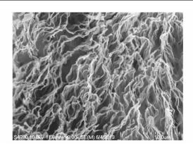
1,2,3,4-Erythrityl tetranitrate (ETN) was prepared by using erythritol as raw material, fuming nitric acid and concentrated sulfuric acid as nitrating agent and catalyst respectively. Its micro morphology, structure, thermal decomposition, detonation performance and sensitivities were studied by optical microscope, scanning electron microscope (SEM), X-ray diffraction (XRD), differential scanning calorimetry (DSC) and sensitivity tests.
