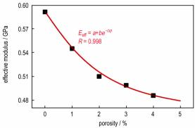
Finite Element Modeling (FEM) model of TATB based polymer bonded explosive (PBX) with microstructure similar to the true one were obtained by a representative volume element (RVE) method. Two-dimension RVE, considering the fraction and distribution of the fillers and pores was established. Effects of pore structure parameters (pore size, pore space distribution and porosity) on the effective elastic modulus of TATB based PBX were analyzed.
