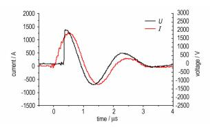
HUANG Na, TANG Hong-pei, HUANG Yin-sheng, HE Yi Chinese Journal of Energetic Materials, 2014, 22(4): 514-520 The electrical explosion performances in three kinds of exploding foils Cu, Cu/Au and Cu/Al/Ni were studied by designed test circuit.
