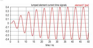
BAI Ying-wei, REN Wei, LIU Ju-peng, ZHONG Jian-wu Chinese Journal of Energetic Materials ,2014 ,22(4): 521-524 To get the response rules and some important parameters affecting the EED response, the relationship between the induced current and frequency in the electromagnetic environment of electro-explosive device was studied by using a continuous electromagnetic wave environment simulation system and an induced current testing device.
