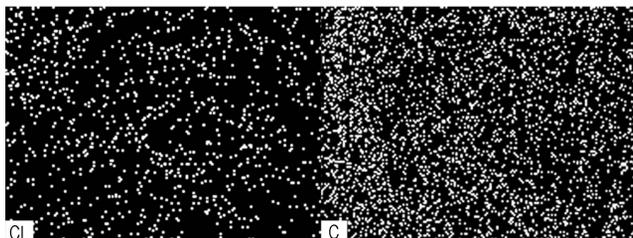
Fig. 2 Distribution of elements Cl and C for HMX/AP/EP composite
