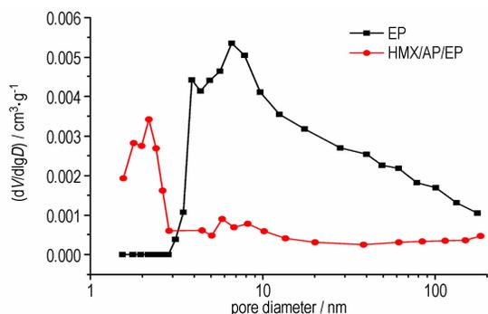
Fig. 3 The pore-size distribution of EP and HMX/AP/NBC composite
