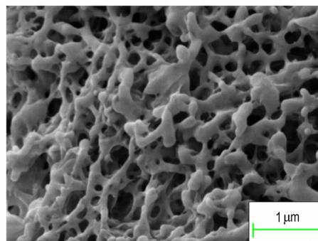
Fig. 1 SEM image of HMX/AP/EP composite
