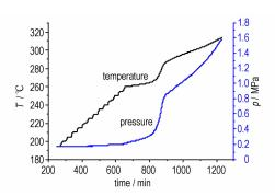
The adiabatic decomposition process of TANPyO was studied by accelerating rate calorimeter (ARC). Temperature rise rate, temperature and pressure versus time curves, pressure and temperature rise rate versus temperature curves were obtained, respectively. Kinetic and thermodynamic parameters were calculated by temperature rise rate equation and Arrhenius equation.
