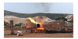
tive consequences was carried out between the fuel tanks with and without explosion suppression infill to evaluate the effectiveness in flame retardant and explosion suppression of the infill. The cook-off experiments were performed on tanks with diesel fuel (-10PD) and with jet fuel (RP-5), respectively, simulating the situation of fuel tanks of vehicles or aircrafts being cooked off. The sizes of the fireballs, the surface temperatures, etc. were recorded.
