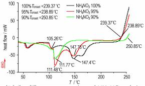
Thermal analysis for different concentrations of  $NH_4NO_3$  solution and 95%  $NH_4NO_3$  solution with different content of  $Fe(NO_3)_3$  were studied by C80 micro thermal instrument in closed environment.
