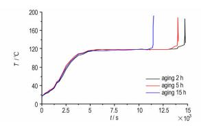
Cook-off test of GATo-3 propellant with different aging degree was carried out by a self-designed device. The self-ignition temperature and self ignition delay period of GATo-3 propellant under the different experimental conditions were experimentally obtained. The related kinetic parameters of GATo-3 propellant were obtained via calculation and the experimental phenomenon were analyzed.
