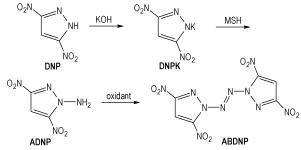
A nitrogen-rich, polynitro energetic compound, 1,1'-azobis(3,5-dinitropyrazole) (ABDNP), was synthesized using 3,5-dinitropyrazole (DNP) as starting material, and its structure was characterized by IR, <sup>1</sup>H NMR, <sup>13</sup>C NMR, MS and elemental analysis.
