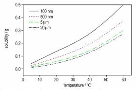
The solubility of RDX with average particle size of 20  $\mu$ m, 5  $\mu$ m, 500 nm and 100 nm in the 8 solvents including the ethyl acetate, ethanol, propyl alcohol, isopropanol, n-butyl alcohol, sec-butyl alcohol, isobutanol and deionized water at 5, 20, 40 °C and 60 °C respectively were studied by the evaporation method of the solvent in the saturated solution.
