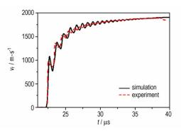
The JWL equation of state of detonation product for CL-20 based pressed composite explosive was researched. The driving ability for C-1 explosive(mass ratio: CL-20 /insensitive binder = 94.5/5.5) was evaluated by 25 mm standard cylinder test. The relationships between expansion velocity/displacement of the cylinder wall and time were studied.
