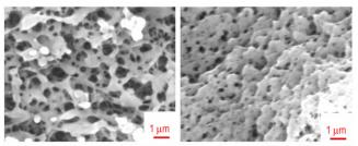
Tow porous reticular HMX, PHMX-A and PHMX-B, were prepared by adding octogen (HMX)/ dimethylsulfoxide (DMSO) complex into pure distilled water or the solution containing polyvinyl pyrrolidone, respectively. Their structures were characterized by scanning electron microscope, X-Ray diffraction, mercury pressure method and thermogravimetry-differential scanning calorimetry.
