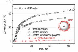
The ultrafine aluminum powders with diameter of  $1-2~\mu m$  were surface grafted by energetic glycidyl azide polymer (GAP) using diisocyanate as bridge via consecutive condensation reactions between —OH and —N = C = O groups. The surface properties, compatibility with fluorine polymeric binders as well as the resistance to water oxidation of the prepared GAP-grafted aluminium powders were studied.
