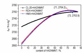
hydroxylammonium 2-dinitromethyl-5-nitrotetrazole (HADNMNT) were calculated by minimum free energy method under the standard condition (ratio of chamber pressure to exit pressure ( $p_{\rm c}$ :  $p_{\rm e}$ ) is 70/1) and the results show that HADNMNT is a potential high energy material in HTPB and CMDB propellants.
