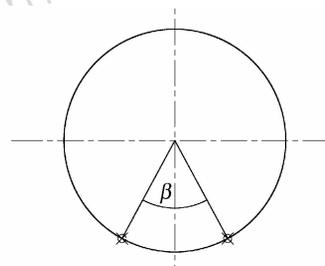
Fig. 11 Layout of two lines initiation
