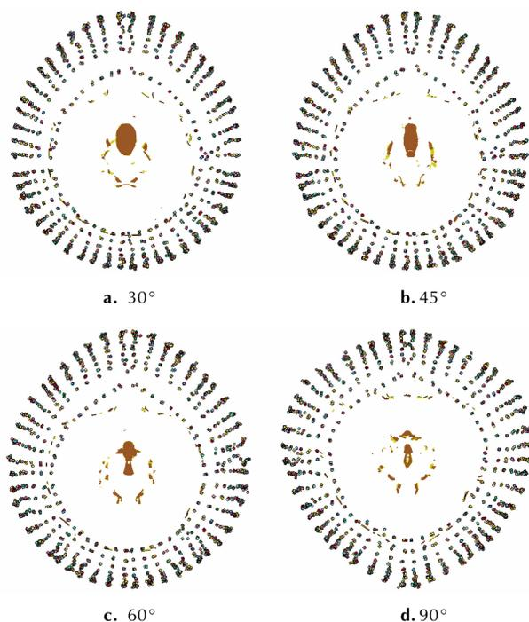
Fig. 16 Fragments dispersion of asymmetrical three lines initiation with different central angle ( $\alpha$ )
