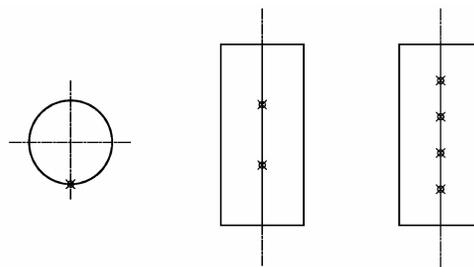
Fig. 7 Initiator layout of asymmetrical one line initiation
