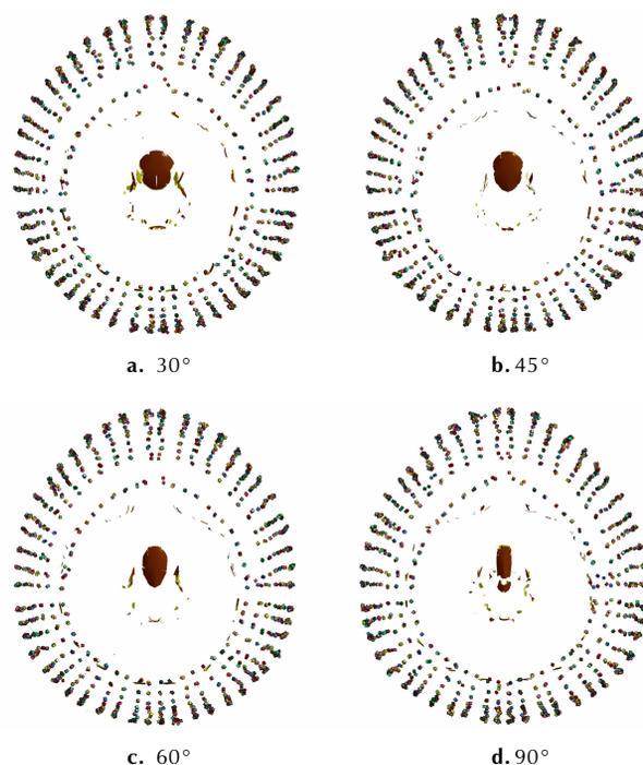
Fig. 12 Fragments dispersion of asymmetrical two lines initiation with different central angles ( $\beta$ )
