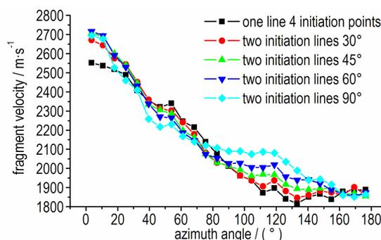
Fig. 13 Fragment velocity distribution along the azimuth angle
