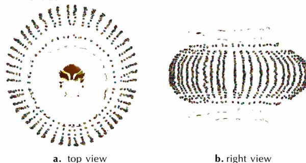
Fig. 8 Typical fragments dispersion of asymmetrical one line initiation
