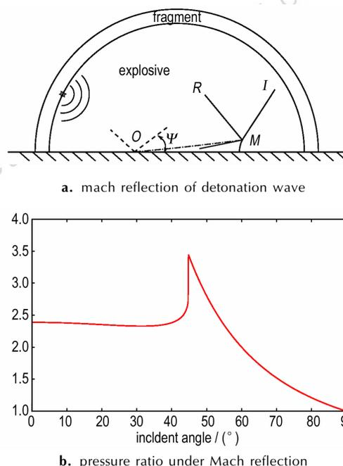
**Fig. 14** Detonation wave reflection
