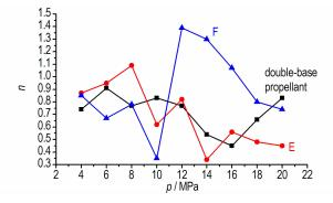
The feasibility of Fe(  $\blacksquare$  ) and Co(  $\blacksquare$  ) energetic complexes of 2, 6-diamino-3, 5-dinitropyridine-1-oxide (ANPyO) as combustion catalysts was tested by closed bomb test and target lines experiment.
