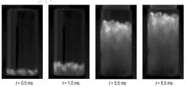
The combustion gas generator and cylindrical filling liquid chamber were designed. The expansion processes of multiple wall jets were recorded by the means of high-speed digital photographic system. The average axial displacements of multiple wall jets at different time were obtained by disposing the expansion sequence diagrams. The effects of the number of orifices and the blasting injection pressure on expansion characteristics of multiple wall jets were discussed.
