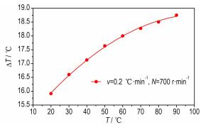
The solubility of HMX in  $\gamma$ -butyrolactone was measured by a laser-monitoring observation method. The relation of the solubility vs. temperature were established. The effects of saturation temperature, stirring speed and cooling rate on metastable zone width were studied. The nucleation series effected by cooling rate and stirring speed were calculated.
