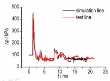
Explosion experiments of thermobaric explosive were implemented in an explosion chamber. Pressure histories were obtained by piezoelectric measurement system. At the same time, the experiments were simulated with AUTODYN. The propagation characteristics of shock wave were obtained by analyzing the pressure-time curves of test and simulation. The curves of overpressure-time obtained by test and simulation were compared.
