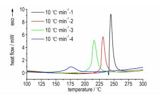
Thermal decomposition characteristics of nitroguanidine (NQ) was studied by differential scanning calorimetry (DSC) dynamic experiment. The effect of thermal history on the thermal stabilities of NQ was investigated by "interruption and re-scanning" method, and the conclusion was verified with the isothermal DSC experiment. The adiabatic security of NQ was investigated by the adiabatic calorimeter (ARC).
