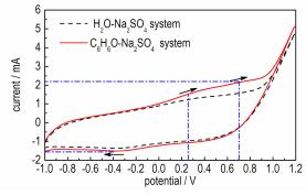
The oxidation of phenol onTi/IrO2-Ta2O5 electrode mainly occurs in the range of oxygen evolving potential. The electrochemical reaction behaviors of phenol on Ti/IrO2-Ta2O5 electrode were investigated by cyclic voltammetry. The efficiency of the electrode degradation of phenol was explored.
