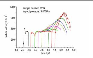
Al-based electromagnetic particle velocity gauge together with gun driven experimental technique were studied. The reaction-build-up velocity profiles of HMX-based explosive with high accuracy under four different incident shock wave pressures are obtained by the Al-based electromagnetic particle velocity gauge.
