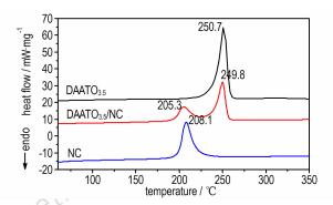
The interactionand compatibility of *N*-oxidiation-3,3'-azobis(6-diamino-1,2,4,5-tetrazine) (DAATO<sub>3.5</sub>) with main components of modified composite double-base(CMDB) propellant ware studied by using differential scanning calorimetry (DSC) and vacuum stability test (VST) method, and the compatibility of DAATO<sub>3.5</sub> with mixture system of CMDB propellant was investigated by curing experiment of propellant at 70  $^{\circ}$ C.
