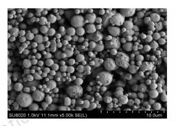
$\rm HMX/F_{2602}$  core-shell composite microspheres were prepared via coat of  $\rm F_{2602}$  on HMX particle surface using the suspension spray drying method. The effects of the suspension spray drying technological conditions including the inlet temperature, feed rate and solution concentration on the particle size of  $\rm HMX/F_{2602}$  core-shell composite microspheres were investigated.
