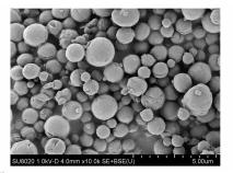
The spherical micron HMX particles were prepared bythe spray drying
