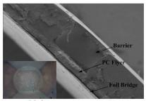
Photolithography and CVD techniquesare employed to fabricate an integrated EFI with Parylene C flyer and Su8-2150 barrier. The Photonic Doppler Velocimetry is also been adopted for the parameter research of integrated EFI's performance, the result seems that the velocity characteristic profile of the integrated EFI is similar to the one fabricated with polyimide flyer and steel barrier. In addition the HNS-IV is successfully been detonated by the integrated EFI.
