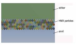
Two-dimensional numerical simulation of the impact process for drop hammer on granular HMX was carried out by using ANSYS/AUTODYN software. The temperature rise generated in particles was estimated via the principle converted from plastic work to heat energy based on the calculated values of stress and plastic work.
