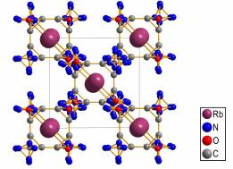
A new green energetic material dirubidium 5,5'-bis(tetrazole-1-oxide) (BTORb) was synthesized and characterized.
