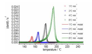
Thermal decomposition characteristic of nitroguanidine (NQ) was studied by dynamic and isothermal differential scanning calorimetry (DSC). Friedman method was used to obtain the activation energy under both mode. The kinetic parameters were settled by model fitting method, and the single step autocatalytic model was verified by the dynamic data.
