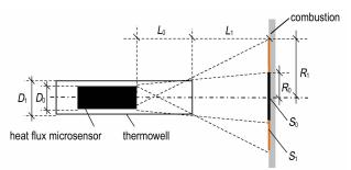
The measurement method for broadband thermal radiation temperature of propellant combustion, was maily accorded to the geometric relations of heat thermal sensor and hermowell, and determined the temperature area and heat radiation receiving conditions. The heat flux value of propellant combustion was measured by using a heat flux sensor, combined with the parameter of test system, and the flame surface temperature of measuring area was calculated.
