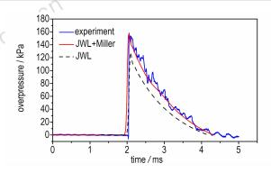
The cylinder test with diameter 25 mm and some static explosion experiments were carried out. The parameters of Jones-Wilkins-Lee (JWL) equation of state were obtained by the cylinder test, JWL-Miller model was introduced to simulate the propagation process of shock waves of thermobaric explosive (TBE). The curves of overpressuretime obtained by experiment and simulation were compared.
