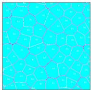
Periodic representative volume element models were established to predict the effective elastic modulus of PBX. According to the mesostructure of polymer bonded explosives (PBX), irregular polygonal particle models based on Voronoi method were established, which achieved extremely high particle volume fraction (over 85%).
