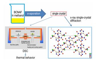
A new energetic compound 4,4'-bis (chlorodinitromethyl)-3,3'-azo-furazan was synthesized as an important intermediate. Its structure was firstly confirmed by X-ray single-crystal diffraction. The thermal stability was determined by thermo-gravimetric analysis (TG) and differential scanning calorimetry (DSC).
