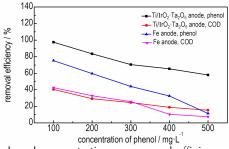
The effect of phenol concentration on removal efficiency were investigated with  $\rm Ti/IrO_2$ - $\rm Ta_2O_5$  and Fe as anode.
