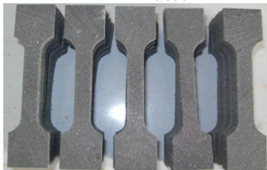
Fig. 1 HTPB solid propellant test specimen
