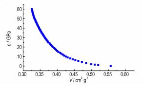
Based on the self-consistent force field-phonon (SCFF-phonon) approach with the anharmonic effect, the isentropic compression loading locus for  $\alpha$ -RDX was obtained, covering a full pressure range (i.e., ambient to the high pressures at von Neumann spike) to which the explosive are suffered from.
