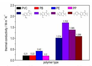
Based on the analyses of the structures, properties, and thermal conduction mechanism of conjugated polymers, several energetic conjugated polymers are designed by introducing energetic group -NO<sub>2</sub>, -N<sub>3</sub> and-ONO<sub>2</sub> on the conjugated polymer structures. The thermal conductivities of new designed energetic conjugated polymers are calculated by Askadskii's group contribution method.
