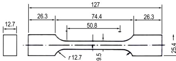
Fig.1 Uniaxial tensile JANNAF testing specimen (unit in mm)
