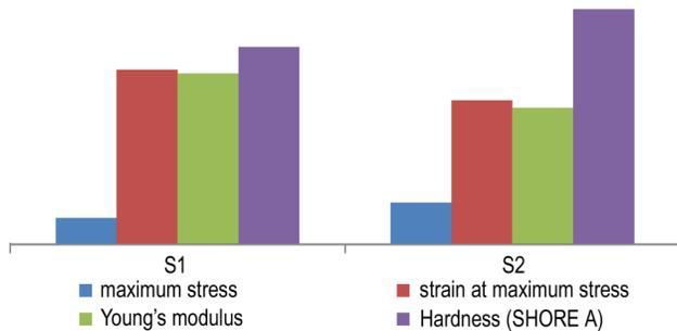
Fig.3 Effect of plasticizers on the prepared propellant samples
