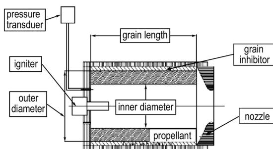
Fig.2 Test stand for the 2-inch motor technique
