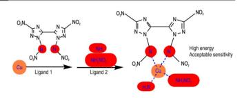
Three new nitrogen-rich energetic complexes Cu(DNABT)  $(NH_3)_{2,x}(NH_2NO_2)_x(x=0,1,2)$  with high energy and acceptable sensitivity were designed by coupling mixed ligands *N*, *N'*-dinitroamino-bi(1, 2, 4-triazole) (DNABT) and NH<sub>3</sub>/ NH<sub>2</sub>NO<sub>2</sub> with copper.
