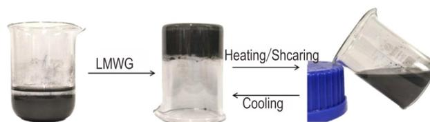
Gelled Al/JP-10 fuels were synthesized using LMWG and aluminum nanoparticles. The basic physicochemical properties of gels such as density, viscosity, volumetric heat and physical stability were compared with pure JP-10. The effect of LMWG and Al on rheological properties of gels were investigated.
