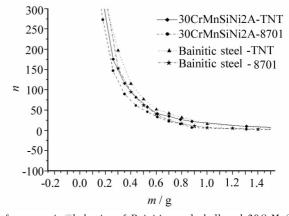
The fragmentation behavior of Bainitic steel shell and 30CrMnSiNi2A steel shell has been studied under the explosive loading. The results show that the initial velocity of the fragments with Bainitic steel shell is higher than that of 30CrMnSiNi2A steel and the fragment number with bigger mass formed from Bainitic is more than that of 30CrMnSiNi2A. Bainitic steel is a better ammunition material coupling with explosive.
