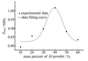
To the mixture dust of Al and RDX powders, a synergistic effect to the maximum pressure seems to exist between the two powders in a proper ratio.
