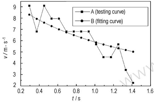
Fig. 3 Relation between rate in the horizontal direction ( $v$ ) and time ( $t$ )
