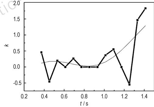
Fig. 4 Curve of the change direction of air friction coefficient ( $k$ ) versus time ( $t$ )
