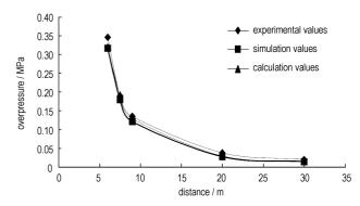
Using the Arbitrary Lagrangian-Eulerian (ALE) algorithm, the numerical simulation of the blasting warhead exploding in the air was realized.
