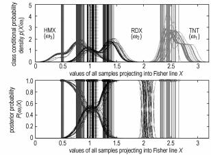
The distinguishing patterns of three explosives (TNT, RDX, HMX) were obtained from GRB images of explosion fireball.
