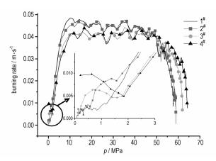
The burning rate of B/KNO<sub>3</sub> was investigated by using closed bomb test system.
