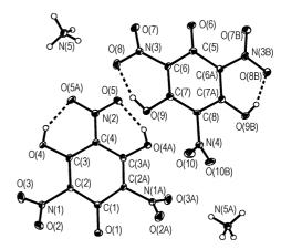
The new compound mono-ammonium trinitrophloroglucinolate was synthesized and characterized. Its crystal structure and thermal properties were determined.
