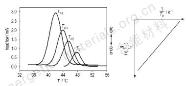
A calculation formula of treating the peak temperature of non-isothermal DSC curves under different constant cooling rate condition was presented.
