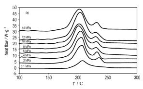
The characteristic values of PDSC( ≤14 MPa) and pressure were correlated to burning rate using an empiric equation by binary regression.
