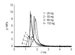
The ignition performances of short impulsive, thruster on different ignition composition amount condition were analyzed through the p-t curves.
