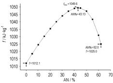
HE Zeng-di, LIU You-ping, HE Li-ming, XIAO Zhong-liang Chinese Journal of Energetic Materials, 2009, 17(2): 202 - 205 The effects of ammonium nitrate on energy of gun propellant were studied. The energy parameters of the gun propellant were calculated. The specific energy, covolume and explosion heat of the gun propellant were tested.
