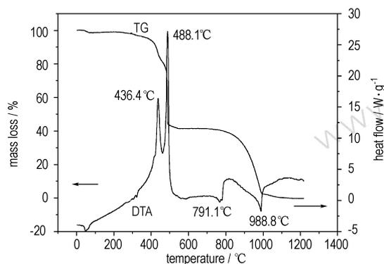
Fig. 7 TG-DTA curves of fog aerosol ( $\beta = 10 \text{ }^\circ\text{C} \times \text{min}^{-1}$ )
