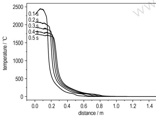
Fig. 4 Comparison of curves of air mass temperature vs distance
