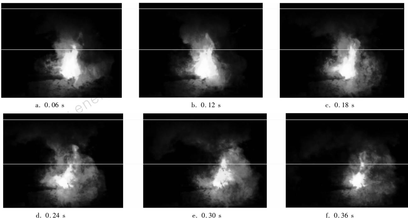
Fig. 2 Diffusion processes of hot air mass produced by combustion of fog aerosol
