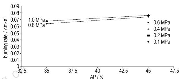
Fig. 4 Effect of the oxidizer solid loading on the burning rate
