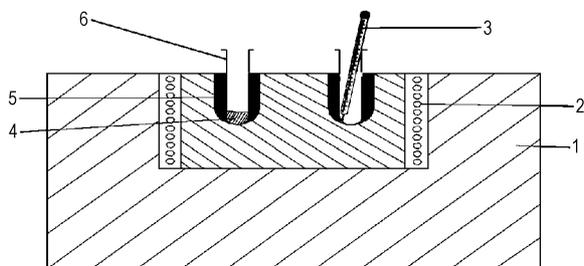
**Fig. 1** Schematic diagram for ignition temperature measurement 1—metal block, 2—controlled heater, 3—thermometer, 4—propellant sample, 5—wood's metal, 6—glass test tube
