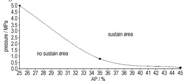
Fig. 2 Effect of oxidizer solid loading on the propellant flammability limits
