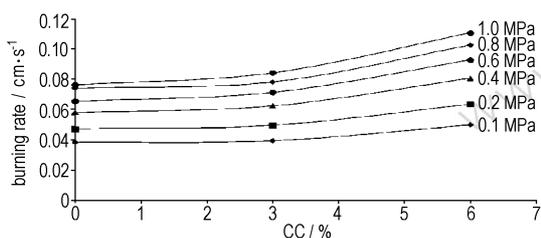
Fig. 6 Effect of the CC solid loading on the burning rate
