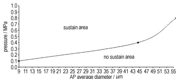
Fig. 3 Effect of oxidizer particle size on the propellant flammability limits
