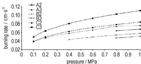
Fig. 7 Burning rate versus pressure correlations for the propellant formulations
