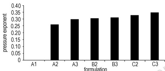
Fig. 8 Propellant formulations effect on pressure exponent
