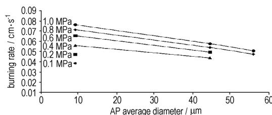
Fig. 5 Effect of the oxidizer particle size on the burning rate
