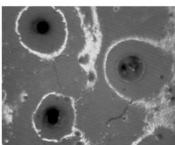
End surface of multiperforated propellant were coated by epoxy resin composite material. On the basis of research on the relationship between opening ratio and the composition of epoxy resin composite material, the opening ratio is up to 99% as the mass ratio of epoxy resin composite material are 60% resin, 40% mixed fire retardant, added 10% diluting agent.
