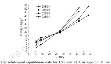
bon dioxide (SC-CO<sub>2</sub>) were measured at different temperature and pressure by UV-Vis. The effects of pressure, temperature and support effect (SE) between molecules of RDX and TNT on the solubility of Chinese Journal of Energetic Materials ,2012 ,20(3): 306 -309 TNT/RDX/SC-CO<sub>2</sub> system were analyzed.
