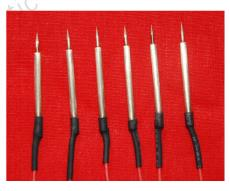
The needle shape probe and corresponding experiment method are designed to measure the precision steady detonation velocity. Results show that the uncertainty of detonation velocity in IHE based on TATB measurement using this electrical pins is not exceed 19 m  $\cdot$  s<sup>-1</sup>, and the relatively uncertainty is not exceed 0.25%.
