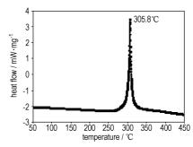
Thermal behaviors of BHN were investigated by DSC and TG-DTG techniques. The compatibilities of BHN with some energetic materials and inert components were examined by DSC method as well as vacuum stability test.
