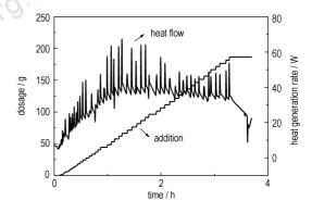
ZHU Yong, WANG Yu, LIU Jian-li, LI Pu-rui, ZHANG Zhi-gang Chinese Journal of Energetic Materials ,2012 ,20(6): 735 -738 The heat release law of the synthesis process of ADN was determined by using reaction calorimeter RC1e. The technical process comprises four stages: neutralization, mixing of nitric acid and sulfuric acid, nitration under lower temperature, amination.
