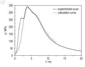
LIU Zhi-tao, XU Bin, NAN Feng-qiang, LIAO Xin, WANG Ze-shan Chinese Journal of Energetic Materials, 2012, 20(6): 701 -704 The simulation of the interior ballistic with standard charge and the low temperature sensitivity coated propellant charge was carried out based on the potential equilibrium theory.
