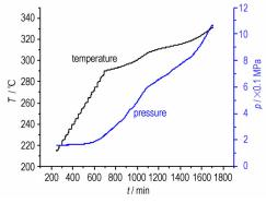
The adiabatic decomposition process of ANPyO was measured by an accelerating rate calorimeter. The decomposition temperature, pressure and temperature rise rate versus time curves, and pressure and temperature rise versus temperature curves were obtained. Apparent activation energy, pre-exponential factor and heat of reaction were calculated.
