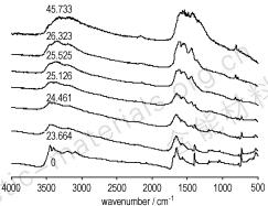
The thermal behavior of guanidinium azotetrazolate (GZT) was studied using the thermogravimetry and differential scanning calorimetry. The thermal decomposition mechanism of GZT was proposed based on the investigation of products in condensed and gas phases by the combination techniques of solid in situ cell with the rapid-scan Fourier transform infrared spectroscopy and pyrolysis-gas-chromatographymass-spectrometry (Py-GC-MS).
