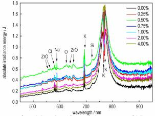
Carbon nanotubes (CNTs) with catalytic property, high specific surface area, strong adsorption capacity and high strength were introduced in Zr/KClO<sub>4</sub> pyrotechnic compound. The effect of carbon nanotubes on the thermal decomposition and light radiation property of Zr/KClO<sub>4</sub>(60/40) pyrotechnic compound used in the pump sources was studied by differential thermal analysis technology and photoelectric detection technology.
