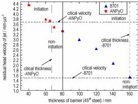
The initiation processes of covered, but unconfined explosives 2,6-diamino-3,5-dinitropyridine-1-oxide(ANPyO) and 8701 by shaped charge with diameter of 56 mm at stand off of 80 mm were studied by jet initiation sensitivity test. AUTODYN numerical simulation method was used to determine the residual head velocity and diameter of jets. The critical thickness of 45<sup>#</sup> steel barrier and initiation threshold of explosives were obtained, and jet initiation sensitivities were discussed.
