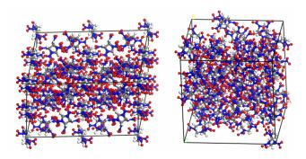
TAO Jun, WANG Xiao-feng, ZHAO Sheng-xiang, DIAO Xiao-qiang, WANG Cai-ling, HAN Zhong-xi Chinese Journal of Energetic Materials ,2016 ,24(4) : 324-330 The cocrystal structure and blending structure with the molar ratio of CL-20 and HMX as 2:1 were constructed. The mechanical properties, structure stability and radial distribution function of the cocrystal system and blending system were simulated by MD method.
