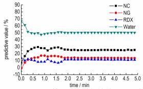
Components quantitative calibration models which were established by NIR spectroscopy were used to analyze the contents of each component and their dispersion uniformity of modified double-base propellant components.
