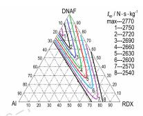
The energy performances of GAP/NC cross-linked double base propellant were predicted, and the iso-property trigonal figures of RDX/oxidizer/Al mass fraction of the propellant with 60% solids content were obtained. The effects of plasticizers and the ratio of RDX/oxidizer/Al were discussed.
