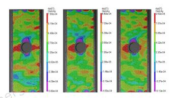
LIU Chen, LAN Lin-gang, TANG Ming-feng, LI Ming Chinese Journal of Energetic Materials ,2016 ,24(4) : 368-374 A tensile test was conducted on a polymer-bonded explosive plate with hole specimen, with digital image correlation method(DICM) applied to analysis the strain fields of the test.
