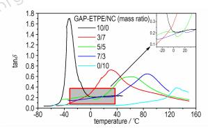
GAP-ETPE/NC polymer blends were prepared using glycidyl azide polymer(GAP) based energetic thermoplastic elastomer(ETPE) and nitrocellulose (NC) with different mass ratios by solution blending process, and their structure, thermal and mechanical properties were investiga-
