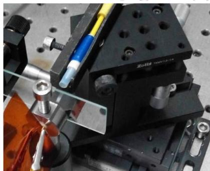
Fig. 4 Picture of EFI assembly on experiment platform
