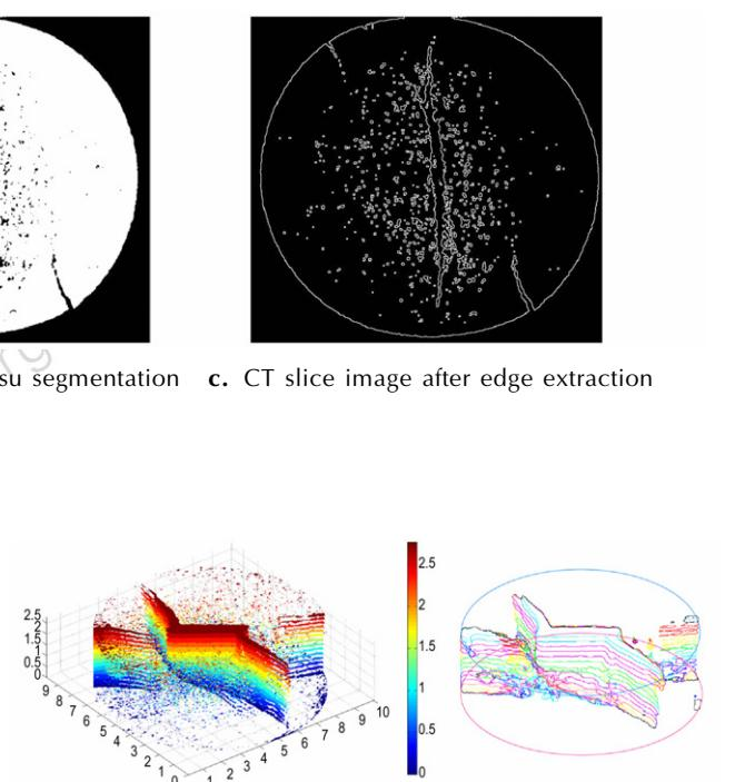
a. 3D morphology and distribution of all cracks and pores      b. 3D morphology of main cracks
