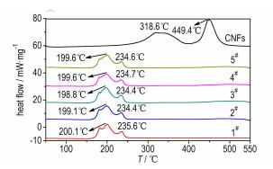
Based on high-energy TEGDN gun propellant formulations, adding a small amount (mass fraction of 0.5%, 1.0%, 1.5%, 2.0%) of cellulose nanofibers (CNFs) obtained from lignocellulose, high-energy TEGDN gun propellants containing CNFs were prepared. The results of TG and DSC show that thermal decomposition performance of high-energy TEGDN gun propellants after adding CNFs is stable.
