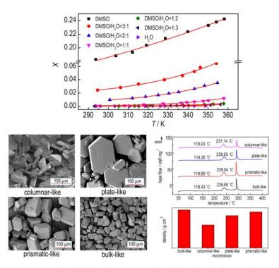
The solubility of FOX-7 in dimethyl sulfoxide (DMSO), water ( $H_2O$ ) and its binary mixed solvent in the range of 20–95 °C and the metastable zone width of binary solvent mixtures DMSO/ $H_2O=2:1$  (in volume ratio) were measured. Crystal characteristics of FOX-7 under various crystallization conditions were investigated by cooling crystallization, and their basic performance parameters test and thermal analysis were carried out.
