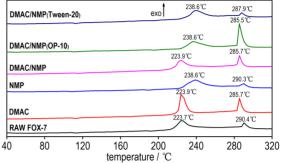
Nano-FOX-7 was successfully prepared by the solvent-nonsolvent method using DMAC, NMP and their mixture. The morphology, phase, structure and thermal performances of the prepared nano-FOX-7 were characterized by FE-SEM, XRD, FT-IR, DSC and TG method and its sensitivities were tested. When using the mixed solvents and adding the surfactants OP-10 and Tween 20 in the solutions, the prepared nano-FOX-7 has better particle size distribution and thermal properties.
