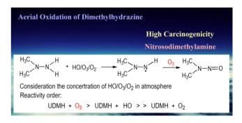
To determine the reaction pathway of UDMH to NDMA in the atmosphere, the reaction mechanism of UDMH oxidation to NDMA in the atmosphere was studied using quantum chemical method. The geometric configuration optimization and frequency calculation of reactants, intermediates, transition states and products of the reaction system were carried out at B3LYP/6-311+G(d,p) and M06-2X/6-311+G(d,p) levels.
