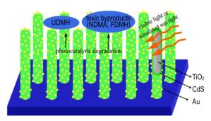
As - prepared TiO<sub>2</sub> nanorod array (NRAs)/CdS/Au thin film photocatalyst was employed to degrade unsymmetrical dimethylhydrazine (UDMH) wastewater under visible light or simulated sunlight irradiation. The degradation of toxic byproducts, nitrosyldimethylamine (NDMA) and hydrazone (FDMH), was monitored during the photocatalytic process.
