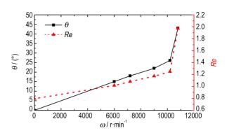
To reserve the micro-scale combustion characteristics of base bleed propellant AP / HTPB under spinning condition, we used the average Reynolds number of the combustion surface to describe the influence of the spinning on the deflection angle of the gas phase flame.
