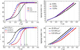
The parameters of elastic/viscoplastic double hollow spherical-shell collapse reaction rate model (DZK) were determined by particle-velocity history curves on different thicknesses of the explosive obtained from the initiation experiment of PBXC03 under the quasi-isentropic loading. Then, the regularities of the initiation process of PBX under quasi-isentropic loadings with different loading slopes and peak pressures were obtained by the DZK model.
