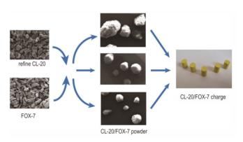
Three kinds of CL-20/FOX-7 PBXs were prepared by water suspension coating method using Estane as coating agent and FOX-7 as energetic sensitivity-reducing component. The morphology, crystal form, thermal decomposition characteristic and impact and friction sensitivity of samples were tested and analyzed by SEM, XRD, DSC, impact sensitivity tester and friction sensitivity tester. The detonation velocity of three kinds of PBXs was tested by an electrical measurement method.
