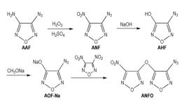
Using 3-azido-4-aminofurazan (AAF) as starting material, a novel energetic compound 3-azido-3'-nitrodifurazanyl ether (ANFO) was designed and synthesized for the first time via Caro's acid oxidation, hydrolysis and intermolecular etherification sequence. The physicochemical properties and detonation performances of ANFO were calculated by DFT method.
