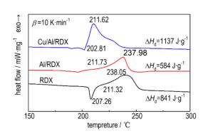
Cu/Al composite was prepared by a displacement method. Effects of the Cu/Al composite on thethermal decomposition of RDX were studied by DSC. The thermal decomposition characteristics of Cu/Al/RDX, Al/ RDX and RDX were also discussed.
